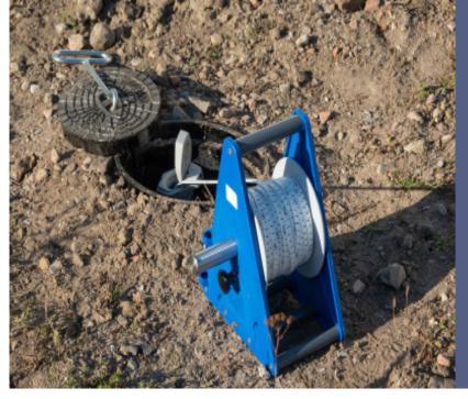
"The difference between high flow and low flow sampling can be seen in the equipment used and the rate at which water is extracted from the ground. These differences are related as different equipment is needed to get water out of the ground quickly."
