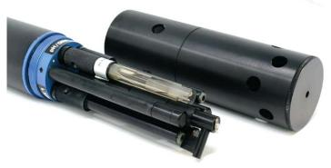
AS-6000 with additional sensors fitted to the body
