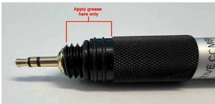
Using a clean cloth or tissue paper, polish the gold contacts ensuring they are completely clean. Carefully insert the electrode into the AUX socket and tighten firmly until the O-ring is completely compressed.
