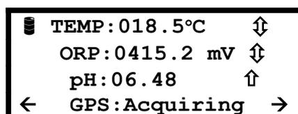
Left/right arrows at the bottom corners of the screen indicate further data screens are available. To access these screens, simply press either the left or right arrow keys. Any value that is out of range or unavailable will be displayed as dashes. The other four screens available with the standard AM-200/AP-2000-D combination are shown below.
