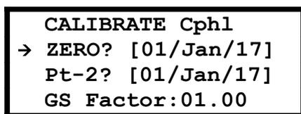
Calibration point 2 (Pt-2) is the upper calibration point.
