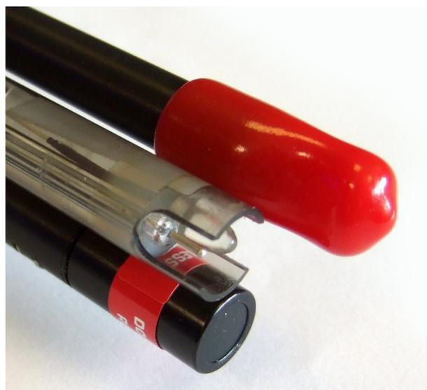
**The caps should be fitted to all ISE Electrodes when using pH calibration solutions or other ISE calibration solutions other than that specific for the ISE being calibrated** in order to protect the ISE electrodes from the effects of the buffer solution and interfering ions.
