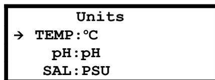
The first option on this screen allows you to change the temperature display between °C and °F.
