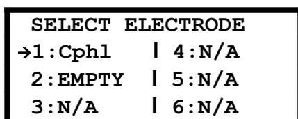
The Cphl electrode should have been assigned to AUX socket 1 when it was fitted. Press the OK or right arrow key to select Cphl. The screen will change to:
