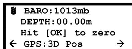
If the depth is not reading zero (this is possible if the probe is wet and a low EC reading is registering), press the OK key. You will be asked to confirm by pressing OK again.
