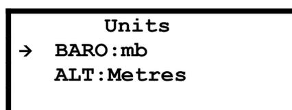
The first line allows you to choose between displaying Barometric pressure in millibars (mb) or in mm of mercury (mmHg).
