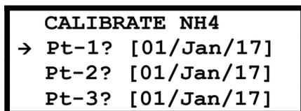
Calibration point 1 (Pt-1) is the warm 10ppm point. Calibration point 2 (Pt-2) is the warm 100ppm point. Calibration point 3 (Pt-3) is the cool 10ppm point.
