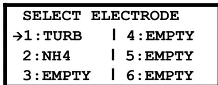
The Ammonium (NH4) electrode should have been assigned to an AUX socket when it was fitted. Move the pointer to NH4 then press the OK or right arrow key to select.
