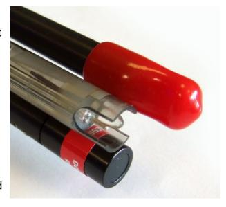
The caps MUST NOT be fitted when calibrating optical electrodes or serious calibration errors will occur due to reflections from the caps.
