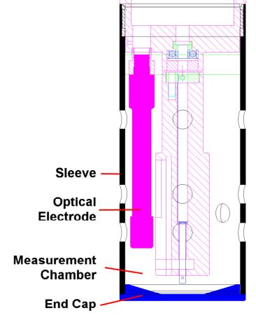
A perfect example of this is calibrating with the end cap removed then measuring with the end cap fitted (or vice-versa). By changing the physical characteristics of the measurement chamber, you also change the calibration and response of the electrode.
