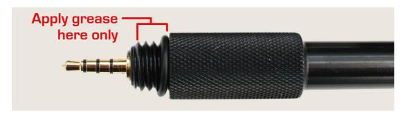
**ENSURE NO GREASE IS APPLIED TO THE GOLD CONTACTS**. Using a clean cloth or tissue paper, polish the gold contacts ensuring they are completely clean. Carefully insert the electrode into the AUX socket and tighten firmly until the O-ring is completely compressed.
