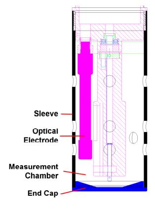
By changing the physical characteristics of the measurement chamber, you also change the calibration and response of the electrode.
