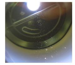
register the equivalent of around 5NTU as each bubble is seen as a solid particle.
