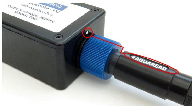
Align the ◀Aquaread® logo on the plug body with white dot on the AP-PC-KIT, then press the plug into the socket and tighten the retaining collar.
