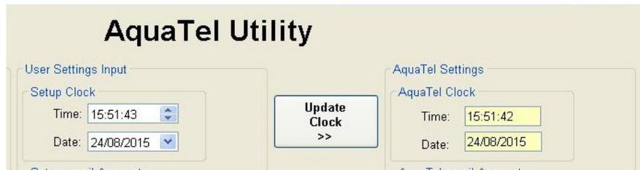
The boxes within the window to the left labelled 'Setup Clock' show the current time and date from your PC. You can override/change this time and date if you want to by directly altering the values within the boxes.
