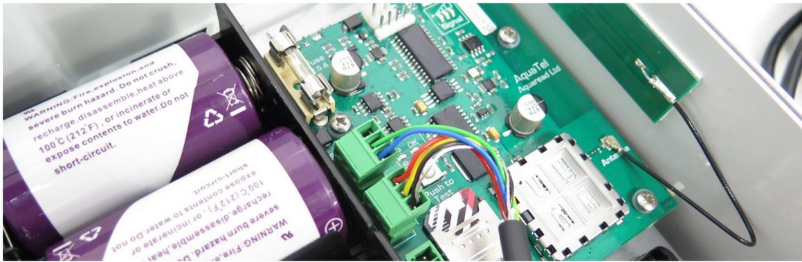
Once the sonde cable has been made off, ensure the cable gland is tightened to prevent water ingress.
