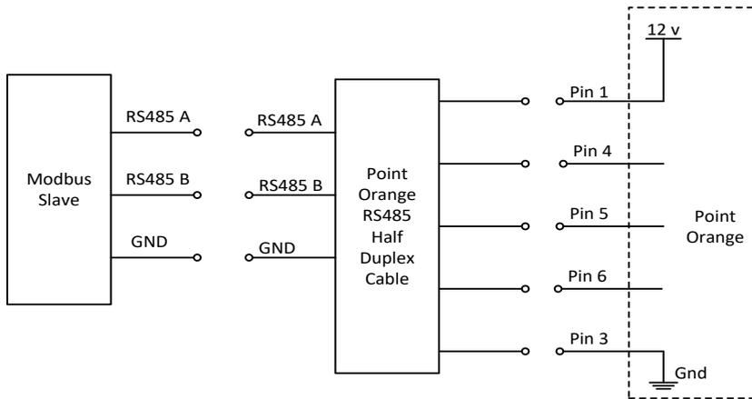
Figure 19: Modbus RS485 Half Duplex connections
