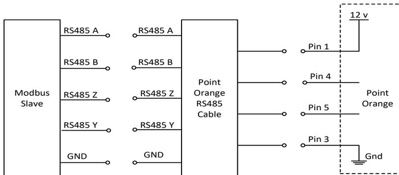
Figure 20: Modbus RS485 Full Duplex connections
