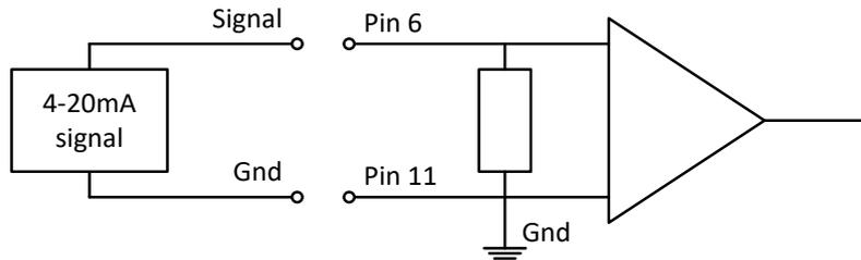
Figure 13: Typical passive loop connections
