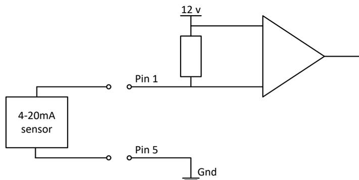
**Figure 9: Typical active loop connections**
