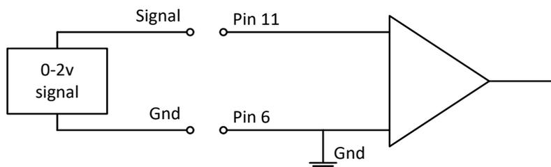
Figure 15: Typical passive voltage connections
