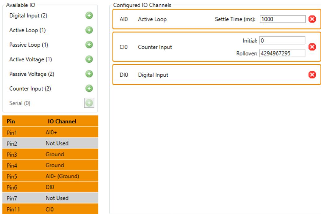
Figure 3: IO Configuration tab
