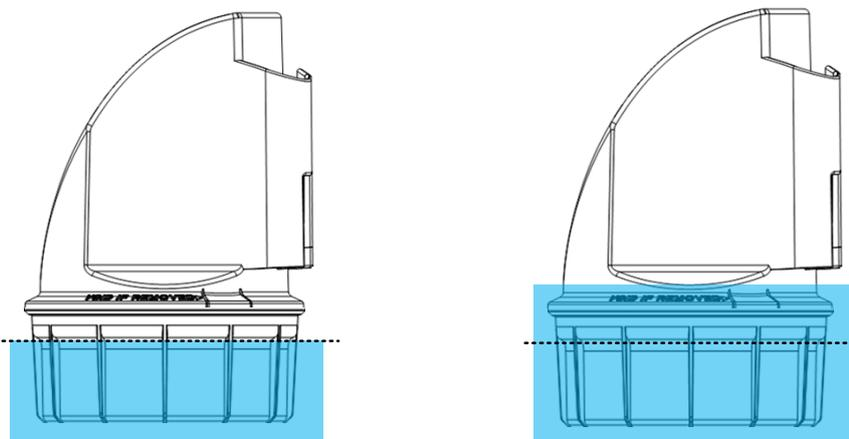
Figure 29: Point Colour submersion threshold
