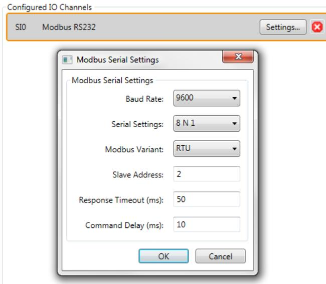
**Figure 21: Modbus configuration**
