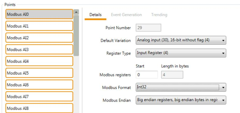
**Figure 23: Modbus register configuration**
