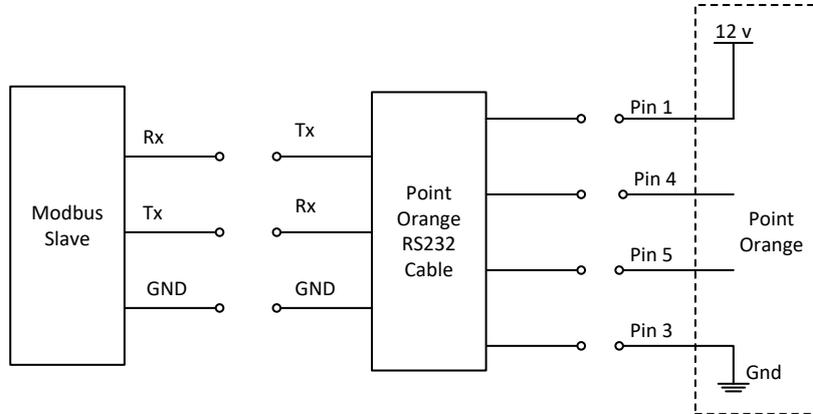
Figure 18: Modbus RS232 connections
