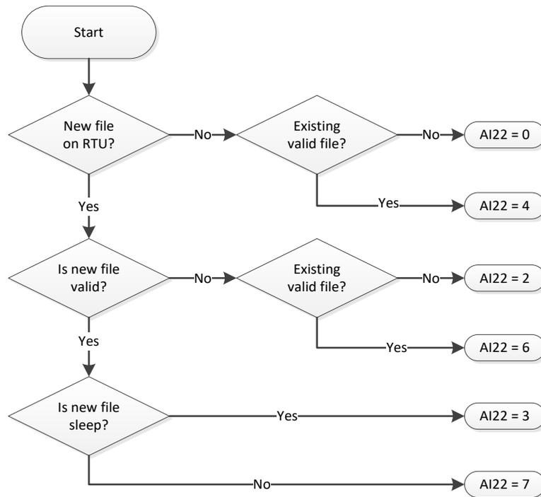
**Figure 41: Flow chart showing the configuration file download states of the Point Colour**
