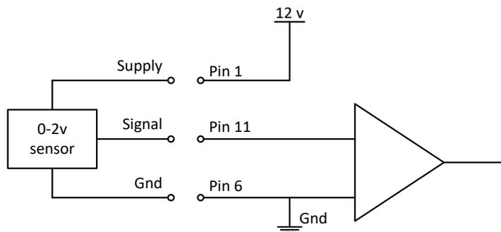
Figure 11: Typical active voltage connections
