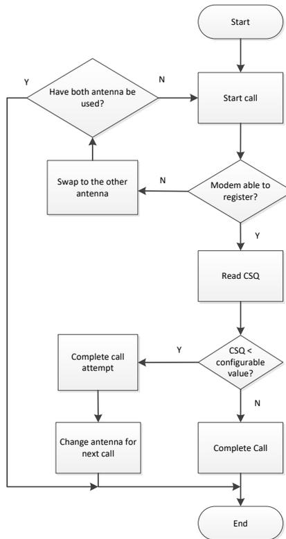
**Figure 39: Automatic antenna selection**
