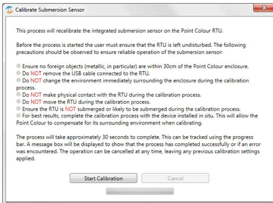
Figure 30: Poco+ submersion calibration
