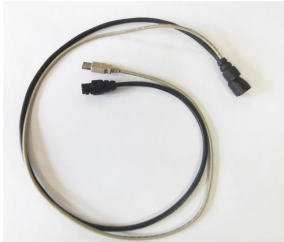
*Figure 40: Programming cable (now standardised to 2m length)*
