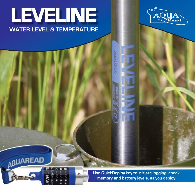
Made from titanium, the new LeveLine is ready for deployment in any environment. It measures water level and temperature for up to 10 years and has a 500,000 dataset logging capacity. Its novel QuickDeploy key and GPS tagging will make both deployment and data analysis easier for you
